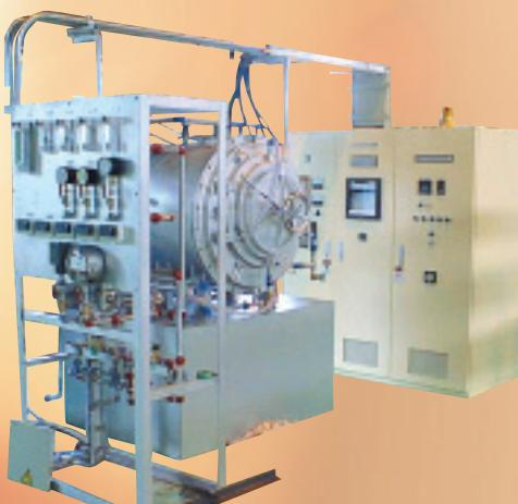
Batch Type Test Firing Furnace
